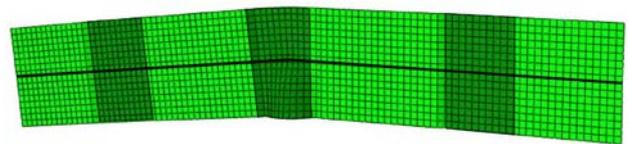
**Fig.5** Ultimate deformation state (Lateral buckling).
