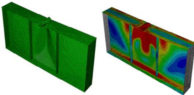
**Fig.15** Case 3 – 50% reduction in THK (For pure bending).
