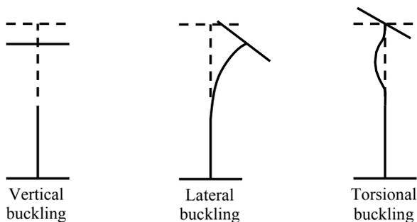
**Fig.2** Buckling modes of plate girders.
