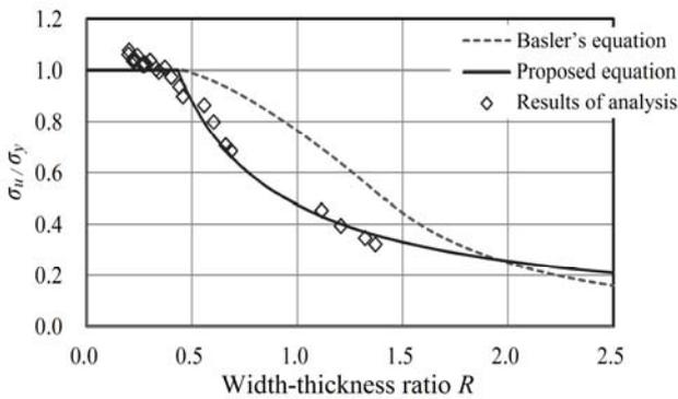
**Fig.9** Load bearing capacity curve (Torsional buckling).
