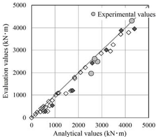
**Fig.17** Comparison of analytical and evaluation values (Bending moment  $M_u$ ).
