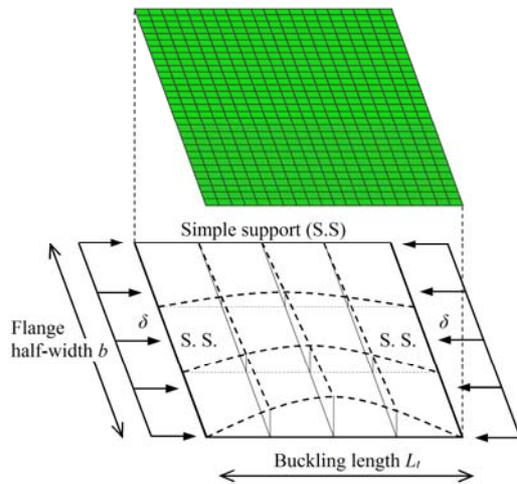
Fig.7 Analytical model (Torsional buckling).
