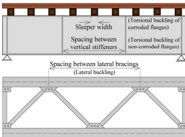
**Fig.3** Basic buckling length of girders with corrosion under sleepers.
