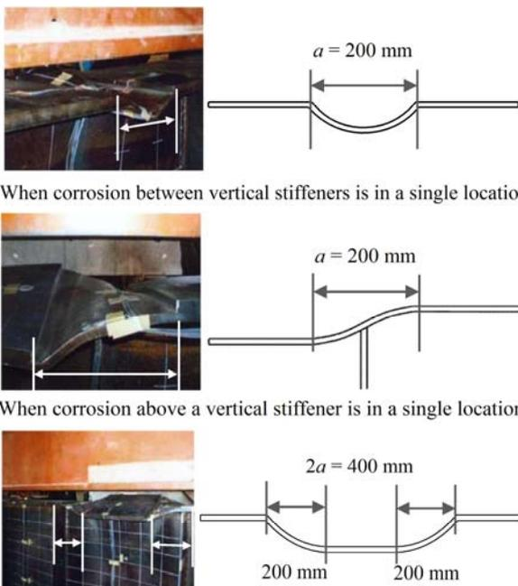
**Fig.10** Way of thinking about buckling length  $a$ .
