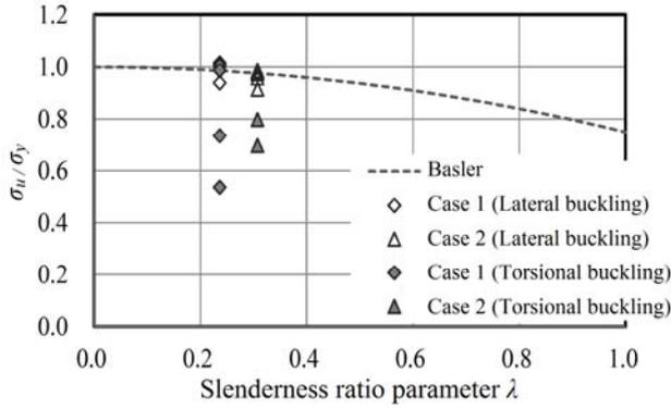
Fig.6 Load bearing capacity curve (Lateral buckling).
