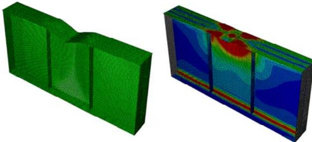
**Fig.14** Case 3 – 50% reduction in THK (For combined load).
