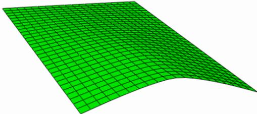
**Fig.8** Ultimate deformation state (Torsional buckling).
